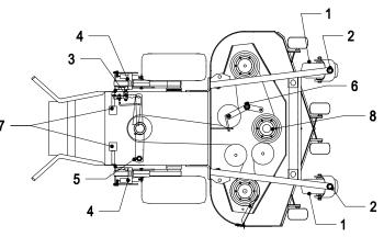
c) Lubricate pivot points with a spray penetrating lubricant as directed below.
